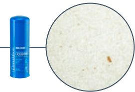
ISO 16/14/11 Target rating for hydraulic/transmission oils
